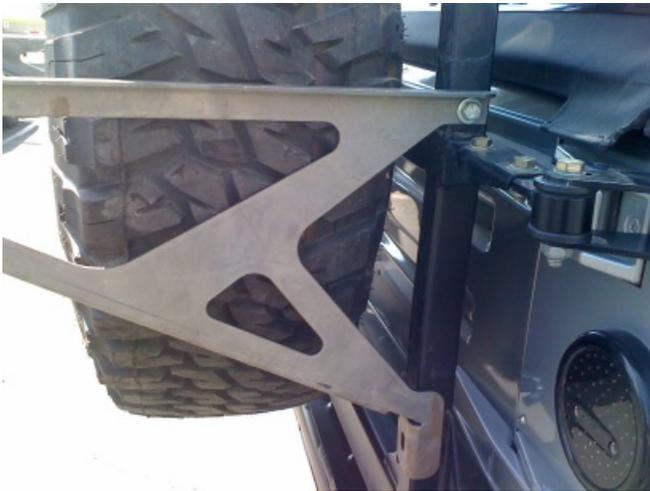
1. Using the supplied L-brackets and hardware, bolt the upper mount to the tire carrier as shown in the photo to the left.
