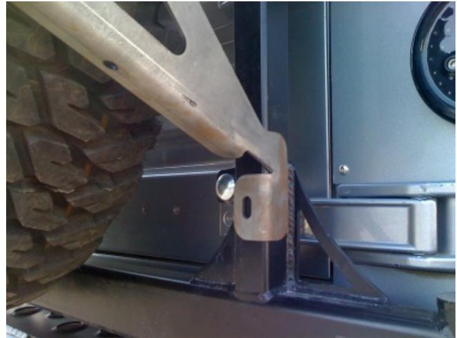
2. With the upper bolt snug, align the lower mount as shown in the photo to the right and drill through the lower portion of the tire carrier for a 3/8" bolt.
